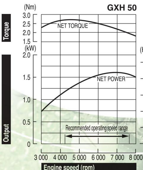
The power rating of the engine indicated in this document is the net power tested on a production engine for the engine model and measured in accordance with SAE J1349 at a specified rpm. Mass production engines may vary from this value. Actual power output for the engine installed in the final machine will vary depending on numerous factors, including the operating speed of the engine in application, environmental conditions, maintenance, and other variables.
